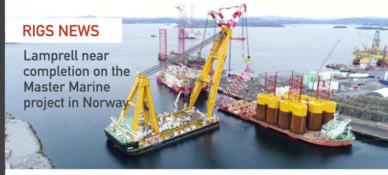
The Lamprell team working on the Master Marine project is close to concluding the "Haven" vessel upgrade after completing all significant construction milestones safely in Norway. The heavy lift vessel "Asian Hercules III" arrived at CCB in mid-January to remove the old upper legs and spudcans from the vessel. Following this in late January, the transport vessel "Mega Trust" delivered the new legs and caissons which Lamprell had previously fabricated in the UAE.
