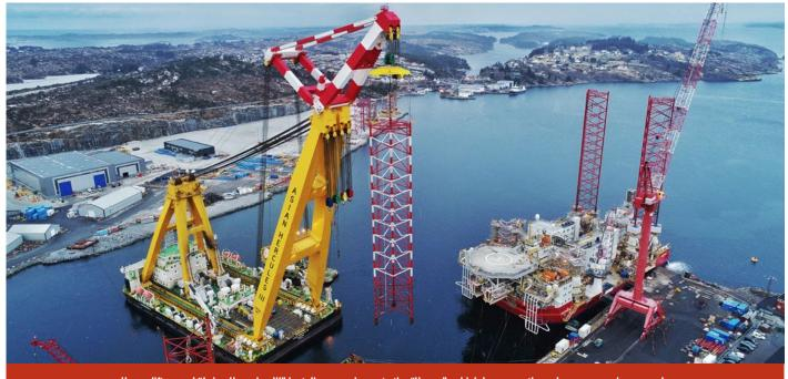
Heavy lift vessel "Asian Hercules III" installs a new leg onto the "Haven", which has recently undergone a major upgrade
