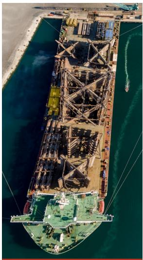
Six flatpack jackets were loaded onto the vessel "Megacaravan 1" in Lamprell's Sharjah facility, and sailed away to its destination in Belfast in December
