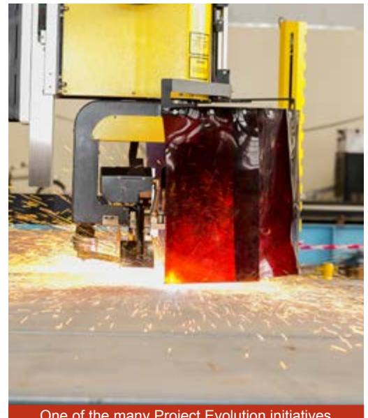
One of the many Project Evolution initiatives to improve cutting capacity is a new plasma cutting machine
