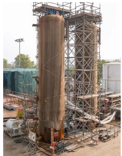
Fabrication is proceeding well for the four molesieve vessels Lamprell are delivering for the Sajaa project in the UAE
