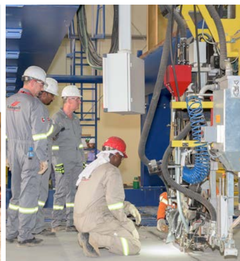
Single sided welding gantry on the panel line
