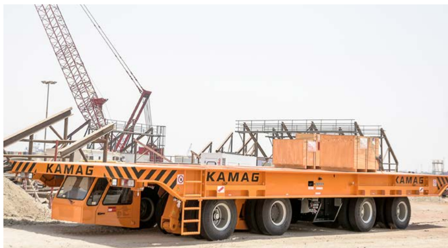
A new Yard Transporter was delivered in July and will provide efficient and low cost movement option for heavy parts and prefabricated sections in our Hamriyah yard
