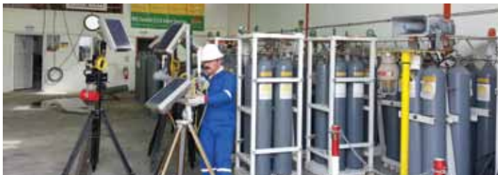
Sunbelt's Sardar Mustafa Saeed testing an H 2 S Wireless Gas Detection system
