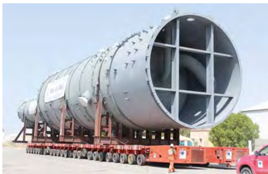
Jacketed pipe units for the Ma'aden Aluminium and Bauxite project for Hyundai / Fluor Worley Parsons
