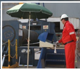
Plate rolling for the caissons on the Master Marine "Haven" project commenced in January in Lamprell's Sharjah facility
