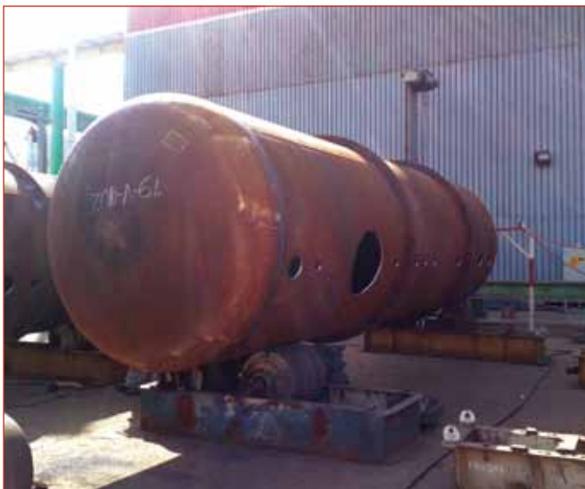
Lamprell is fabricating 20 pressure vessels for Petroserv
