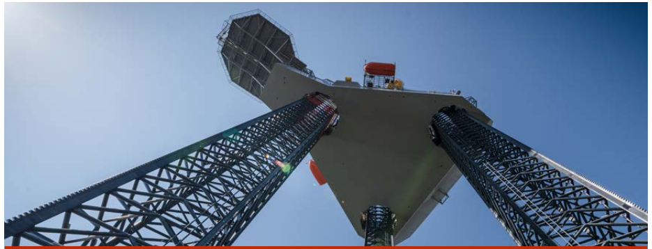
The rig 'Mercury' during jacking trials prior to delivery
